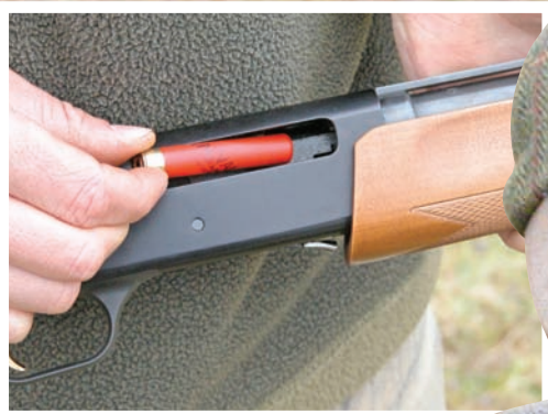
No surprises with the Mossberg 500 action, which uses a skeletonised shell lifter, which makes clearing the occasional stoppage much easier
